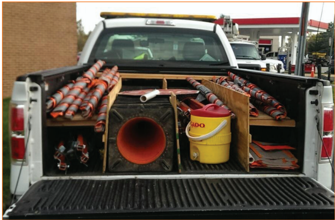
Truck # 13024 Beth Wilson, CL - innovation through load division. Beth installed custom load dividers to keep her load stable and materials easily accessible.
